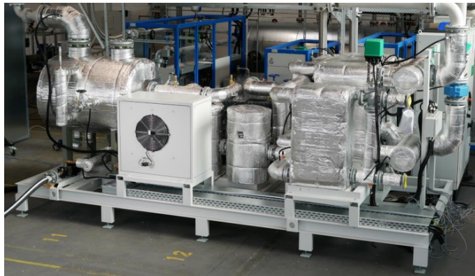
ThermBooster™ with steam generator used in the Gelatine Project
