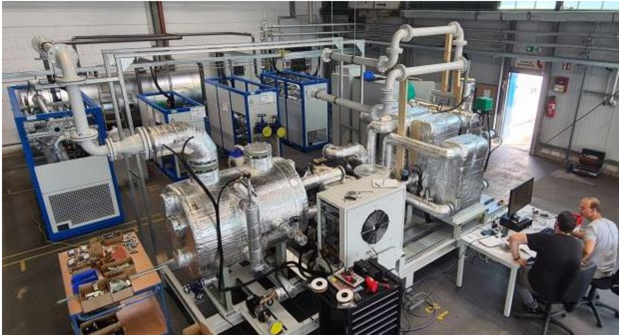
Figure 5 — Installation for the performance testing of the ThermBooster™ in the laboratories of SPH Sustainable Process Heat in Germany.
