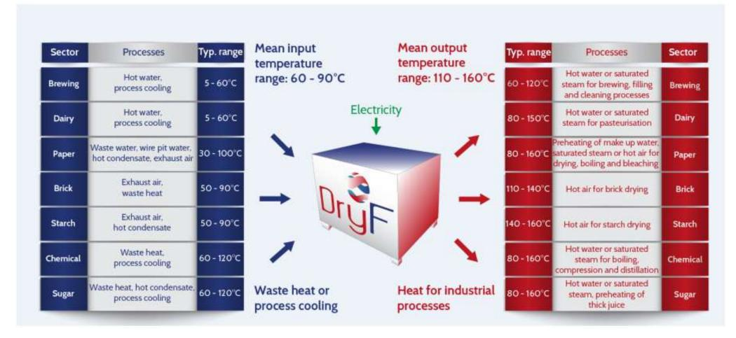
Possible applications of industrial heat pumps (source: dryficiency.eu)
