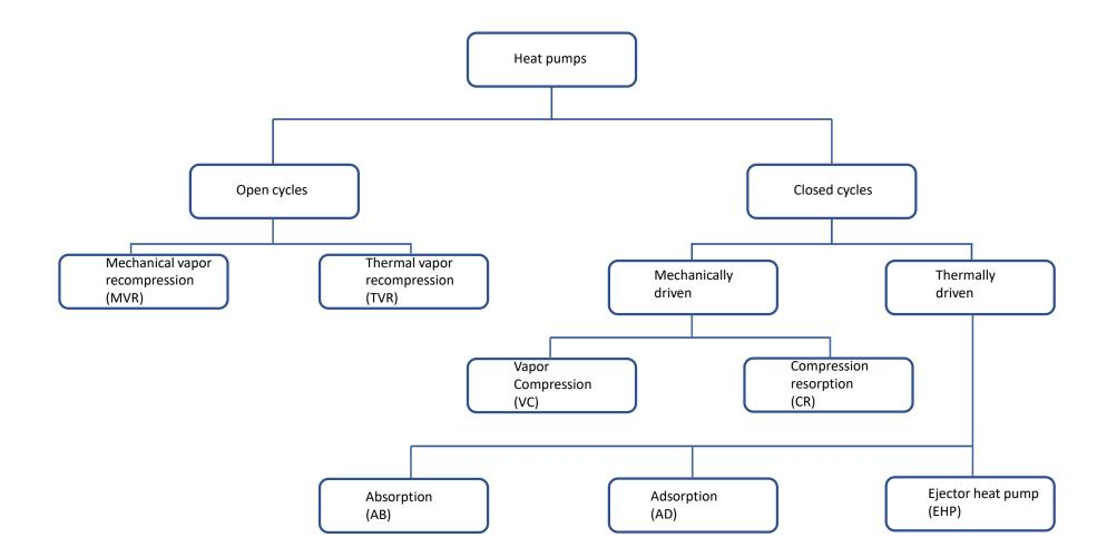
Classification of heat pumps in relation to driving method and degree of being hermetic
