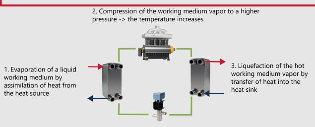
4. Expansion of the liquid working medium to a lower pressure level -> the temperature decreases
