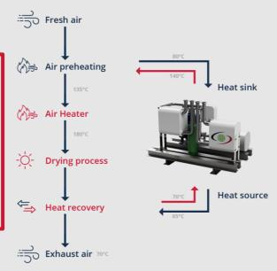
Simplified operation schematics for heat pumps in drying processes.
